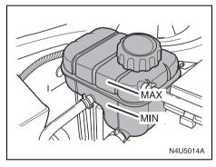
The engine coolant surge tank is located on the driver's side of the engine compartment. See "Engine Compartment Overview" in this section for more information on location.
